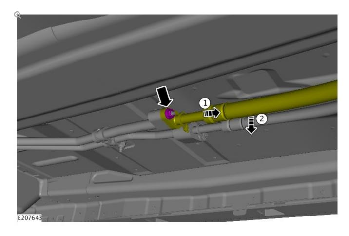
Disconnect the center auxiliary A/C line and check the O-rings for damage.
