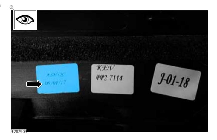
Visually inspect the date printed on the label attached to the new 'A' Pillar finisher.
