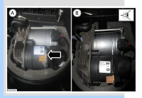
Check for white powder at the suspension air supply unit silencer.
