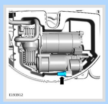
Replace the suspension air supply unit silencer.
