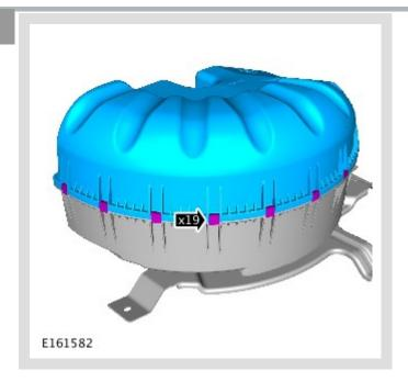
Remove the suspension air supply unit cover.
