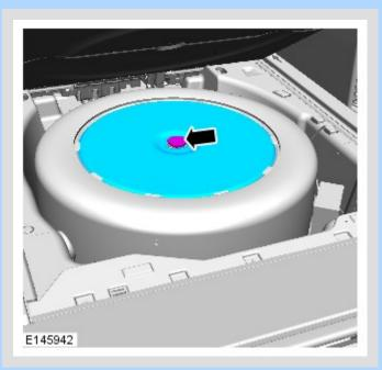
Remove the spare wheel retainer.
