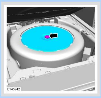
Install the spare wheel retainer.
