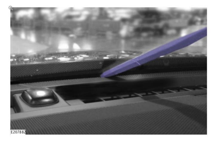
Using a suitable tool, gently open the gap between the instrument panel and the windshield.
