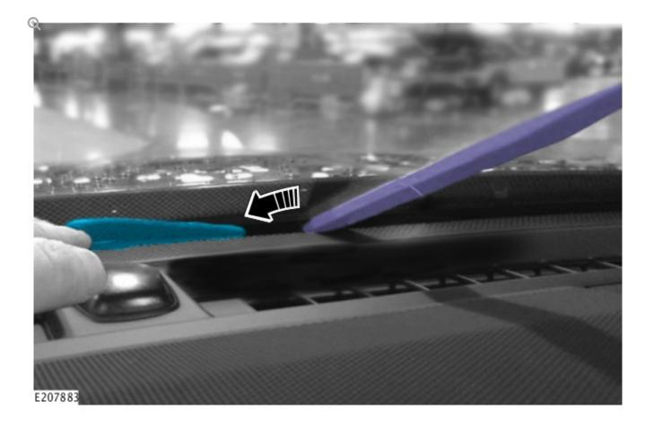
Insert the strip of felt behind the instrument panel center air vent as shown.
