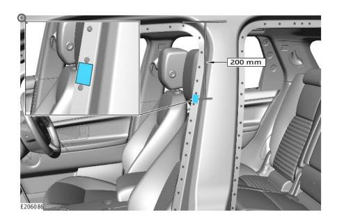
Place a single spot weld within the highlighted area shown.
