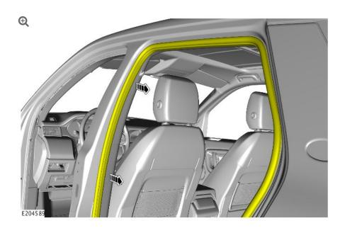
Move aside the rear door aperture seal from the door aperture.
