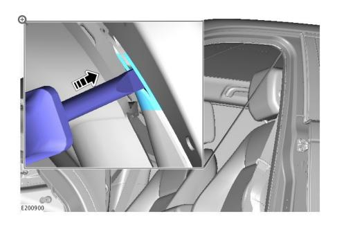
Using a suitable hammer, insert the suitable chisel between the inner 'B' pillar and the cant rail to a maximum depth of 20mm.
