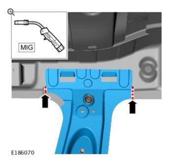
MIG seam weld the 'B' pillar in the area shown. This will eliminate the noise from this area.
