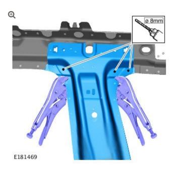
Drill the 3 spot welds to the correct depth of 2.5mm.
