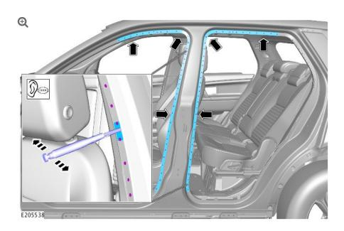
Move the panels, around the door apertures, first inwards and then outwards, as shown until any audible click can no longer be heard.
