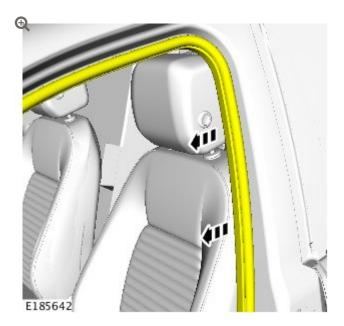
Move aside the front door aperture seal from the door aperture.
