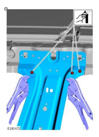
Use a suitable corrosion protection to cover the repaired area.
