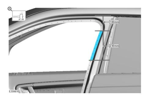
Using a suitable tool, strike the panel with as much force as can safely be applied inwards over the highlighted area shown.
