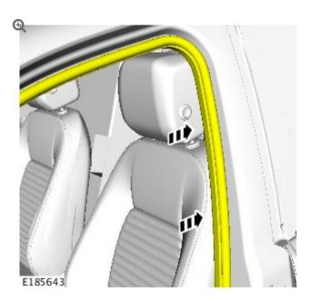
Install the front door aperture seal to the door aperture.
