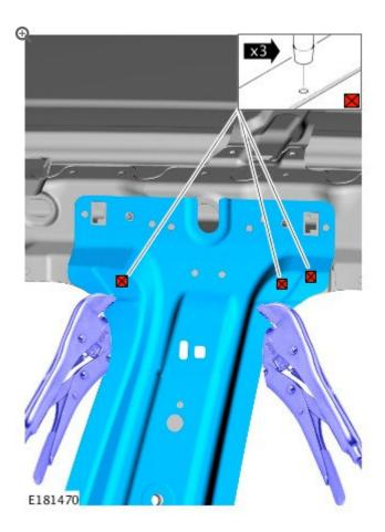
Metal Inert Gas (MIG) weld the 3 drilled holes.
