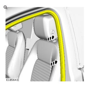
Install the front door aperture seal to the door aperture.
