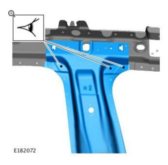
Identify the 3 spot welds to be drilled.
