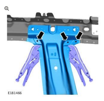
Make sure that when installing the suitable tools to clamp the 'B' pillar the spot welds that are to be drilled remain visible.
