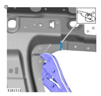
Grind away any excess material where the vehicle has been MIG welded.
