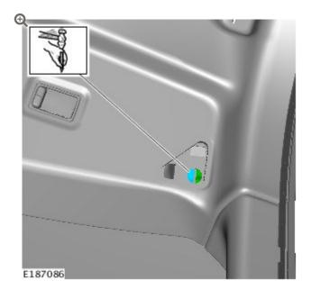
Insert a parallel pin punch with a minimum diameter of 16mm, through the sun visor bracket aperture.
