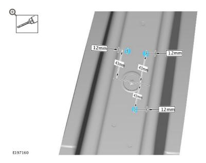
Drill 3 6.5mm diameter holes in the areas shown to a depth of 6mm.
