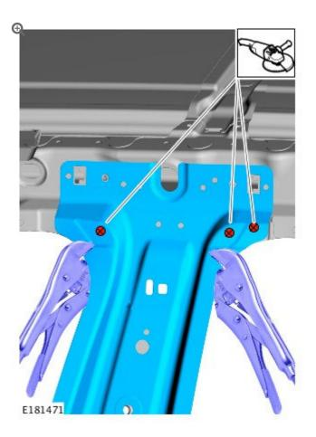
Grind away any excess material where the vehicle has been MIG welded.
