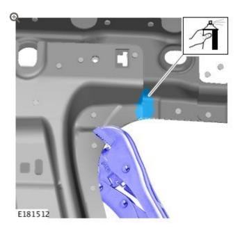
Use a suitable corrosion protection to cover the repaired area.
