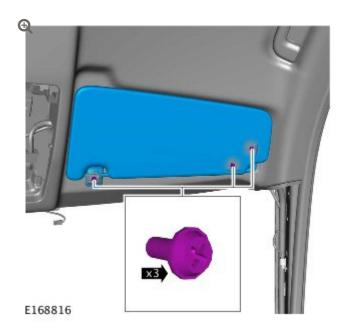
Remove the 3 bolts and remove the sun visor.
