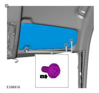
Install the sun visor and tighten the 3 bolts.
