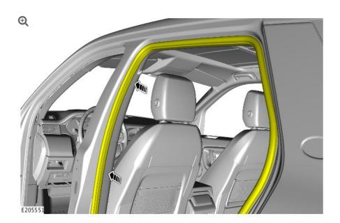
Install the rear door aperture seal to the door aperture.
