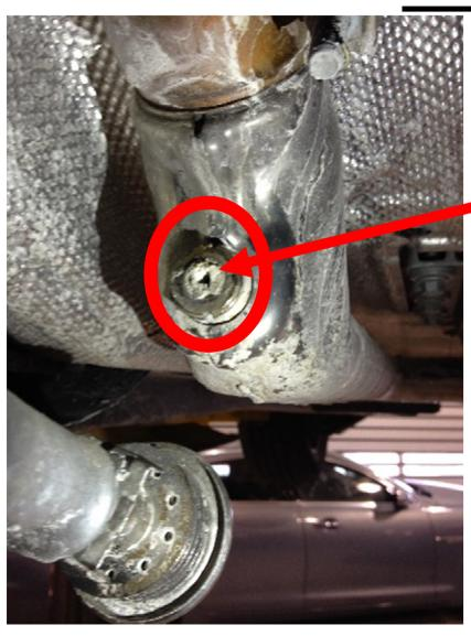
Check for any heavy deposits build-up at the injector seat.
