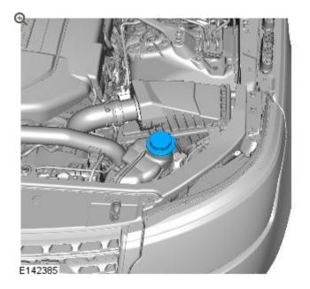
Slowly remove the coolant expansion tank cap from the coolant expansion tank to release the pressure.
