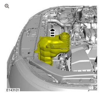
Raise the coolant expansion tank a minimum of 110 mm / 4" from its installed position.
