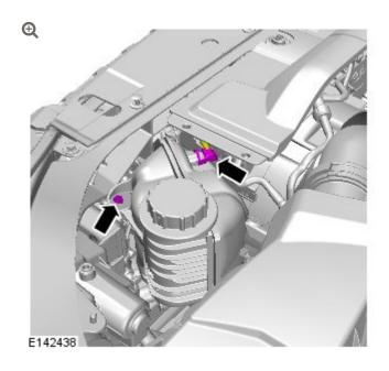
Remove the pipe and fastener from the coolant expansion tank.
