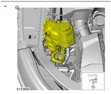
Clamp the hoses to minimize coolant loss.
