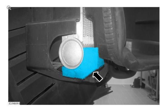
Install the new foam pad to the outer edge of the auxiliary radiator as shown.
