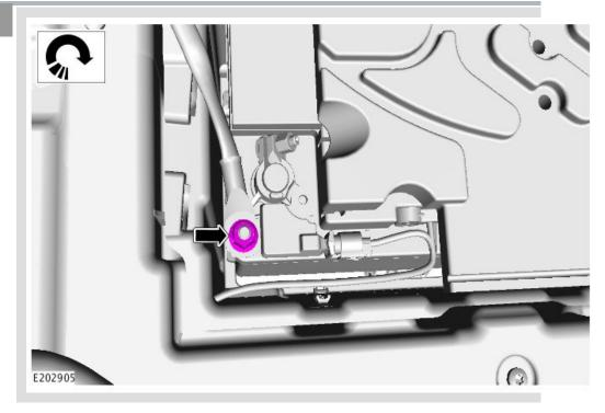
Tighten the nut on the cable connection to the negative terminal bracket.
