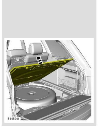
Lift the loadspace board, hook it onto the tailgate opening, and access the spare wheel.
