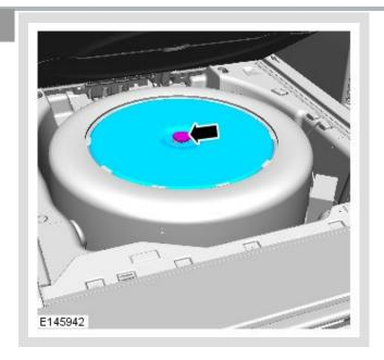
Remove the spare wheel fixing and retainer.
