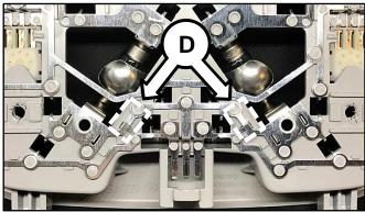
6. Inspect the clearance between each bulb (E) and its reflector (F) and ensure there is a 1mm clearance.
