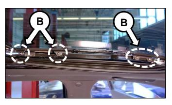
With the assistance of another person, remove the panoramic sunroof glass by sliding the glass towards the front of the vehicle until the sliders are out of the tracks (C).
