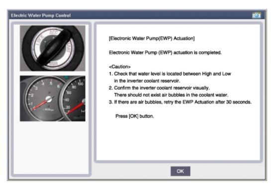
Allow the coolant to settle for another minute. Then run the pump the full run time of 90 seconds and listen to the pump. You can hear a gurgling/sloshing sound if air is still present. If no sound is emitted and coolant circulation without air bubbles is visually verified, bleeding is complete and the message should no longer be present.
