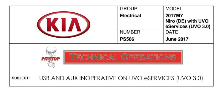
This Pitstop provides information regarding the importance of confirming proper USB/AUX function testing during Pre-Delivery inspection (PDI).
