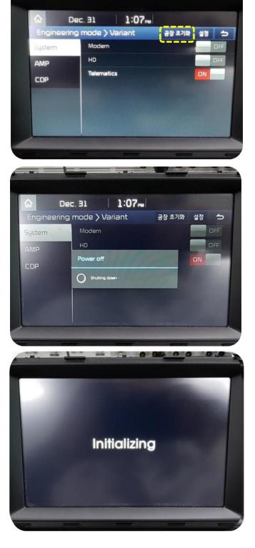
10. The factory reset process is completed after reboot (unit powers off then back on).
