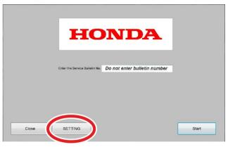
1. Update the PGM-FI or A/T software by selecting the **i-HDS Diagnostic System** icon. Refer to service bulletin 01-026, *Updating Control Units/Modules*.
