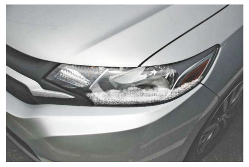
These headlights are semi-sealed and have ventilation holes to help prevent heat deformation. When air flows in and out, however, it also includes any moisture that's in it. If the outside of the headlights are cooler than the temperature inside them, they can fog up.
