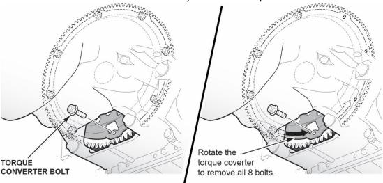
14. Rotate the torque converter clockwise one bolt hole. Then, install the bolts and torque them to 12 N-m (9 lb-ft).
