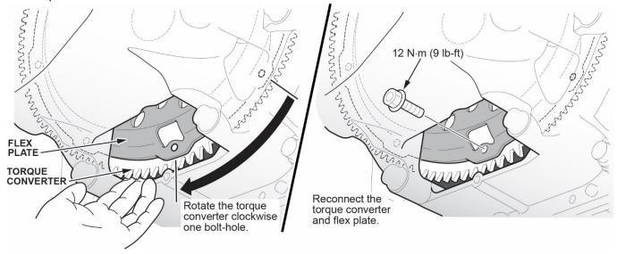
15. Mark the torque converter and the flex plate as shown. Then, write the bulletin number (16-002) on the flex plate with a permanent marker or paint marker.
