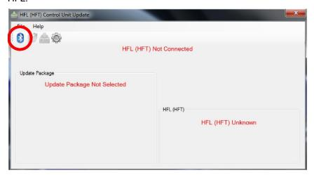
NOTE: If an active *Bluetooth* adapter is not found on the i-HDS laptop, this error message will appear. Review the REQUIRED TOOLS and EQUIPMENT section of this service bulletin for a recognized *Bluetooth* device. Contact your IT support for additional help.
