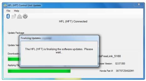
16. In the HFL update tool, click **OK** when the pop-up window indicates the reflash process is complete and the HFL screen indicates the update has completed.
