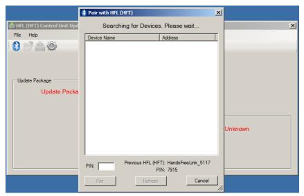
13. In the HFL update tool, once the *Bluetooth* device has been detected, enter the four-digit PIN code from the vehicle's display screen into the lower left hand corner of the pop-up window. Click **Pair** to begin the pairing process.
