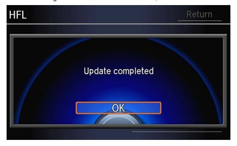
17. The i-HDS laptop will indicate the update is complete and automatically disconnect the Bluetooth connection from the HFL control unit. Close the HFL update tool by clicking the X in the upper right-hand corner.
