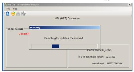
15. In the HFL update tool, the **Open Update Package** window pops up when the *Bluetooth* pairing process is complete. The HFL update tool automatically determines which version of the HFL software is present. The compatible updates will be displayed on the HFL update tool. Click **OK** to begin the HFL control unit reflash process.
