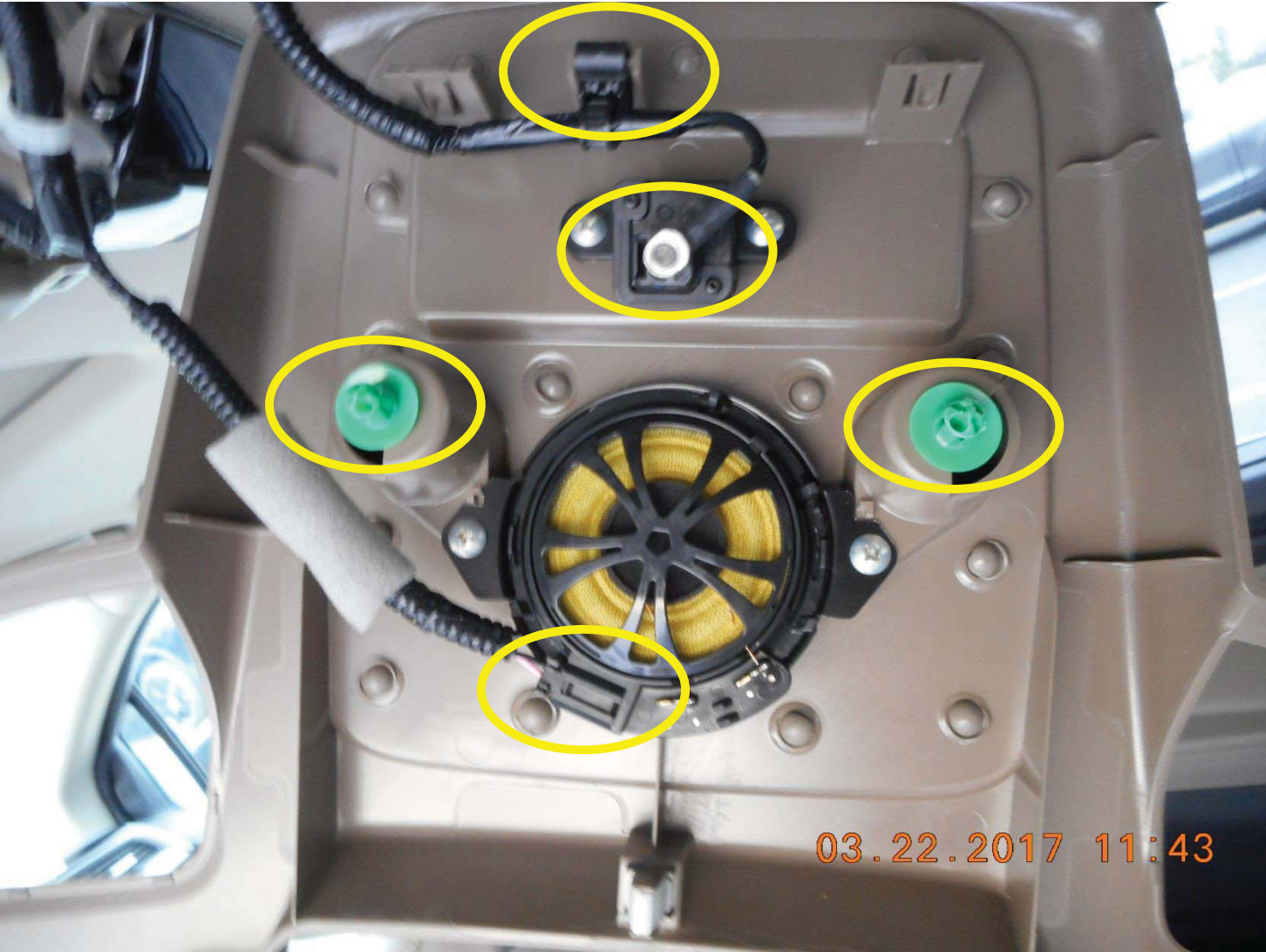
Confirm speaker coupler, green grommets, black camera clip and black camera coupler are secure on display garnish.
