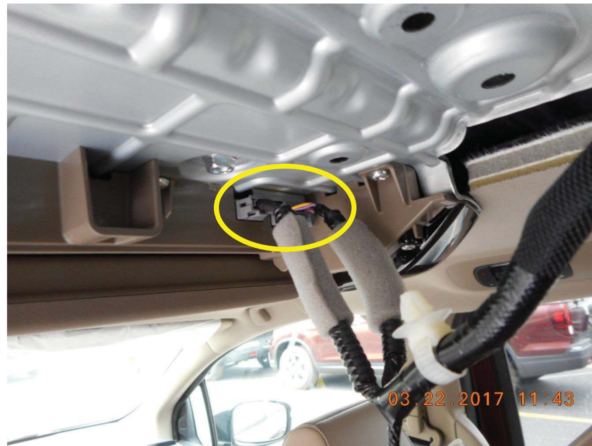
Confirm gray couplers installation by push-pull-push method.
