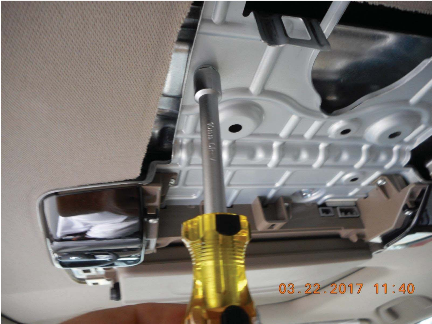
Using 10mm socket reinstall the five 6x12 mm bolts of the new RES Display
