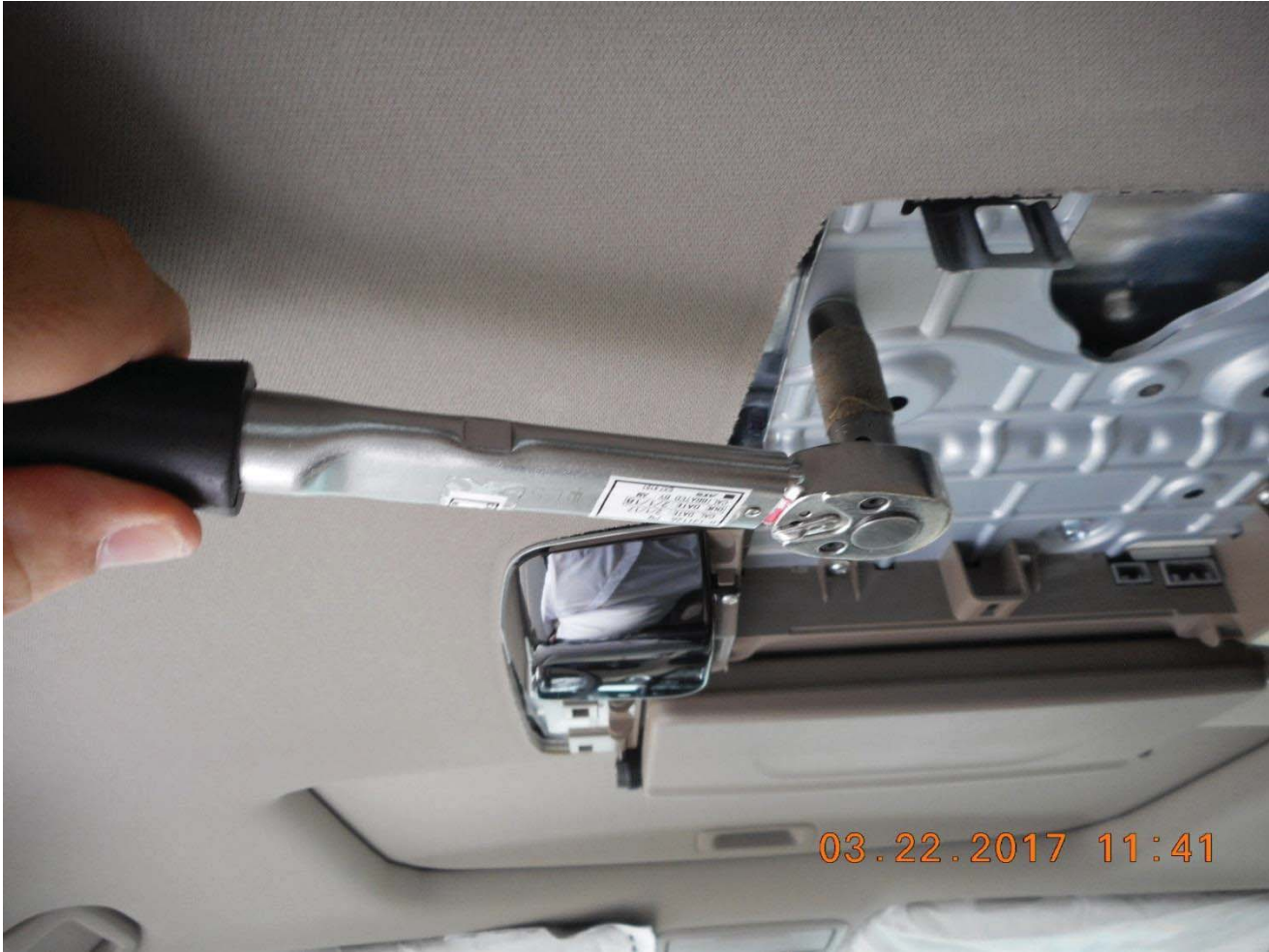
Using torque wrench set at 10Nm with 10mm socket confirm the torque of the five 6x12 mm bolts
