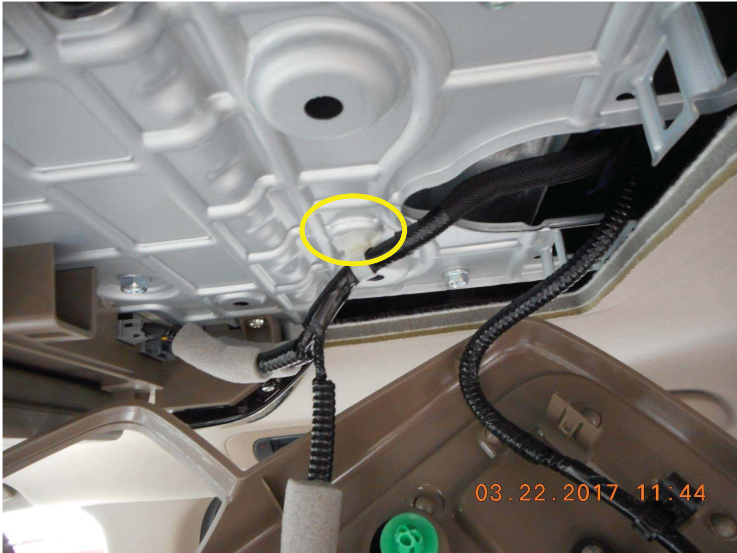
Reinstall white harness clip. Note clip hole is between two larger mounting holes.
