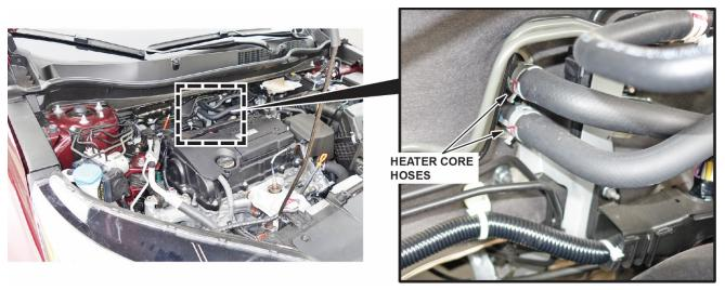
2. Place the new plastic heater clamp on the heater core hoses 10mm from the metal heater core hose clamps. Push the plastic heater clamp towards the rear for a tight fit of the clamp to the metal tube under the heater hoses.
