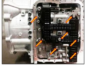
9. Remove two bolts to the upper solenoid support. Remove the support.
