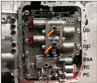
10. Remove the UD solenoid and install a new solenoid.
