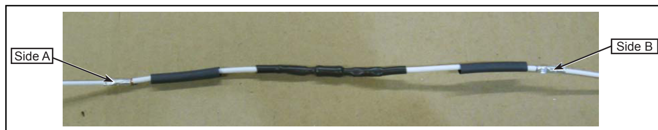
Figure 7 - Typical View of Jumper Harness (N8902748) Connected on Each Side
