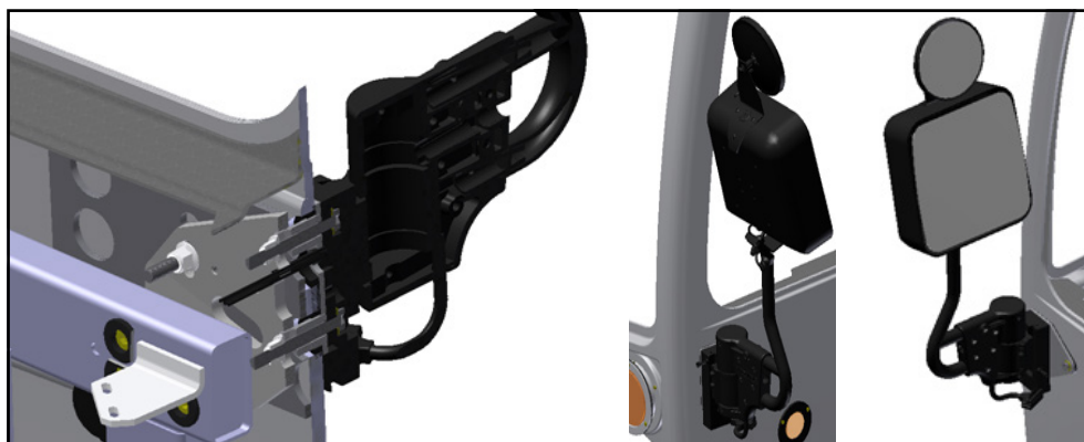
Figure 29 - Installation of Driver's Road Side Mirror Assembly
