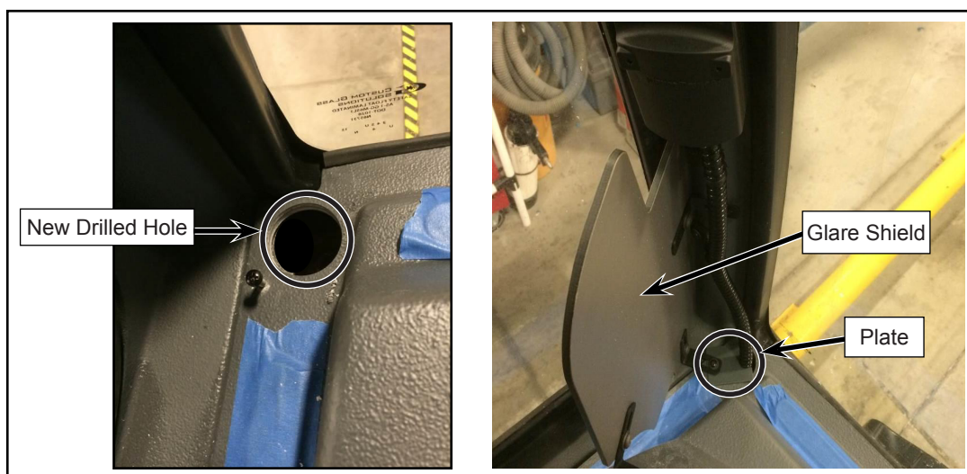
Figure 32 - Installation of Glare Shield and Plate that Covers the New Hole
