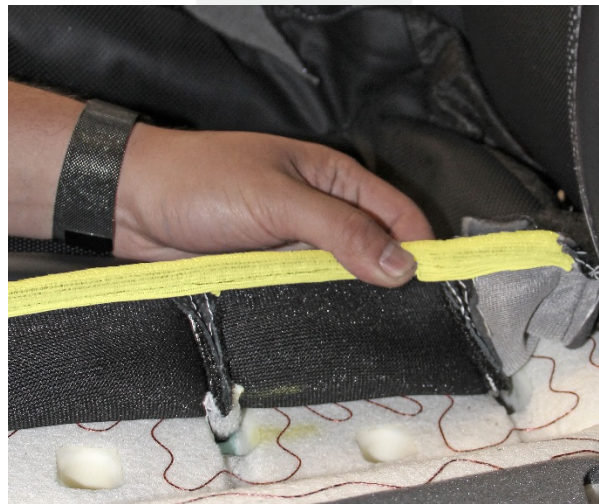
Figure 7 (Hook-and-loop material highlighted in yellow)
