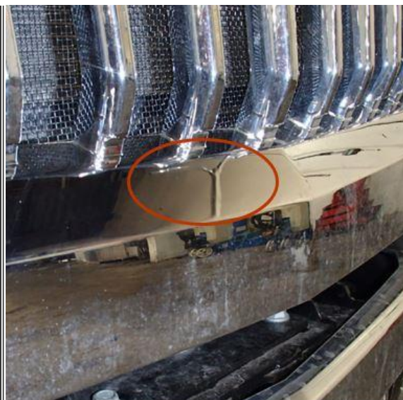
Figure #1: Chrome grille defect
