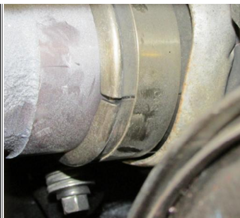
Figure 31: Exhaust Manifold Ring Seal/Clamp
