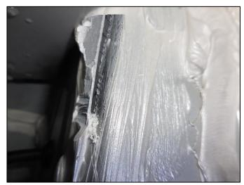
8. Insert the flat screwdriver (P) to pry open about 5mm of the panel opening for seam sealer application.
