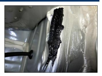
13. After 20 minutes, perform the water spray test noted on page 6 (step 6) to ensure sealant coverage rework is successful.
