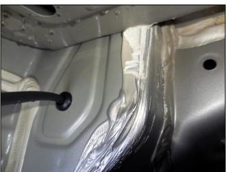
7. Remove 10mm of sealant (N) between the fender apron upper side (L) and front member side (M) using a thin flathead screwdriver (P).
