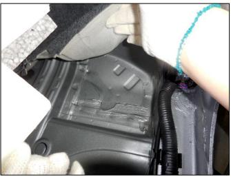
6. Using a hose, spray water directly on the panel opening between the hood, lower pillar and fender for approximately 30 seconds.
