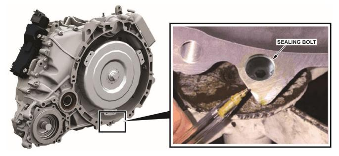
As a temporary fix, the factory installed a sealing bolt in that hole and it's proven effective. That casting issue has since been resolved. Later castings don't have that issue, so there's no need for the sealing bolt.
