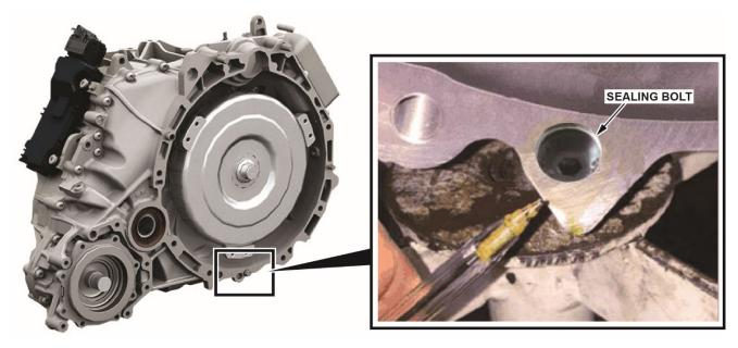
As a temporary fix, the factory installed a sealing bolt in that hole and it's proven effective. That casting issue has since been resolved, and later castings don't have that issue. So, the sealing bolt is no longer needed.
