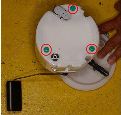
3.) Place the sender/pump module on a flat surface.
