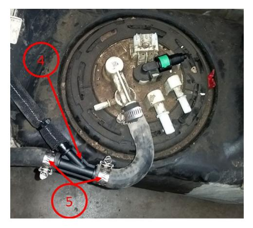
6. It is important to route the Vent Hose over the TOP of the fill hose as seen below (6) to prevent pudding of fuel in the line.
