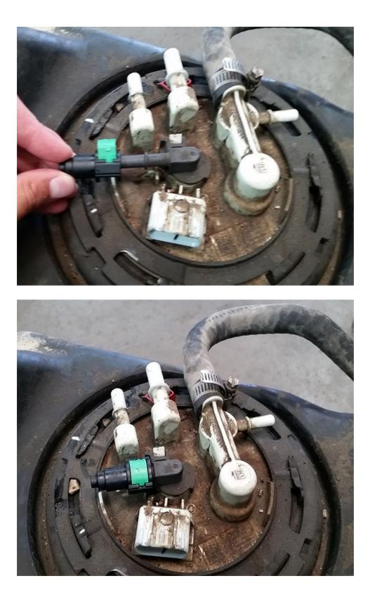
3. Measure the Fuel Tank Fill Vent hose 5 1/2" from the end at the fuel pump module and cut with hose cutters as seen below (2).
