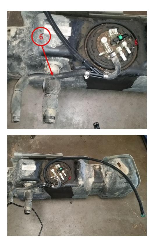
7. Remove the original fuel balance pump line from the pump tube (7) Refer to Plastic Collar Quick Connect Fitting Service. Doc Id# 2147646 and cross member (8) as seen below.
