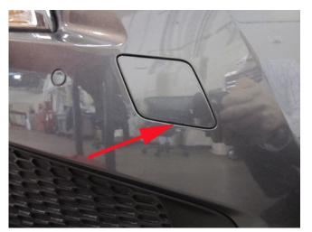
3.2. Carefully open the cover in the front or rear fascia by using the small notch that conceals the tow eye socket. Use care to not damage the paint.
