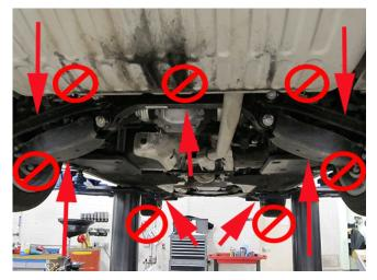
When recovering or transporting a Cadillac ATS or CTS, the under vehicle components may be damaged if the recommended towing and securing steps are not followed.
