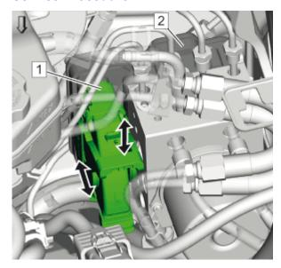
1. Check the pin connection quality and corrosion at the EBCM electrical connector (1).
