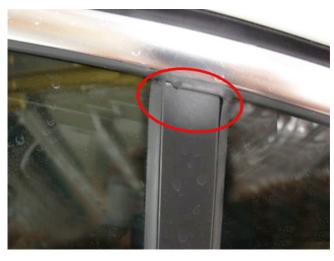
• Inspect the upper division post applique and weatherstrip rubber seal for possible mis-alignment.
