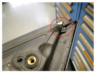
**Note:** The mirror should be installed by the top leading corner first. When installed from bottom corner first, the gasket may catch on the door glass run channel and roll over causing the imperfection shown in the graphic above.
