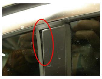
Inspect for a gap caused by the back side retaining clip of the weatherstrip not fully engaged into the door frame.
