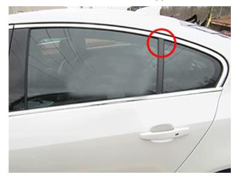
Wind leak cause is most likely gaps at the upper window division post applique and weatherstrip rubber seal.
