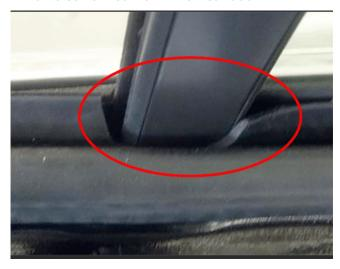
Wind leak cause is most commonly found to be an improperly installed rear side door window inner sealing strip at the lower inner division post.
