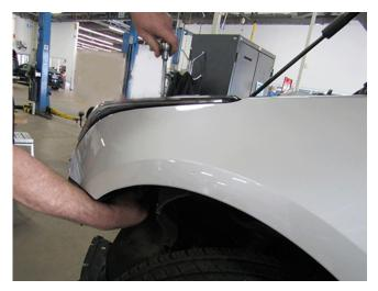
**Note:** Loosely holding the adjuster cable during headlamp aim prevents the cable from twisting, and allows the inner cable to break free from any rust/corrosion.
