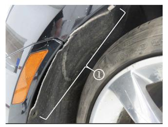
3. Remove the three forward wheelhouse liner fasteners (1) and pull liner away to access the backside of the headlamp. You should be able to tuck the liner behind the tire to temporarily hold it out of position.
