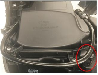
**4.2.** Then pull cable cross-car to unclip the inboard position.
