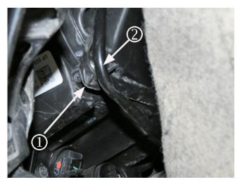
**4.1.** Starting with the outboard clip (1), pinch adjuster cable (2) together and pull rearwards.
