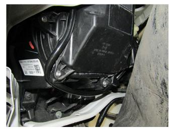
6. Once aim is achieved, reposition the adjuster cable behind the two retaining clips on the headlamp.
