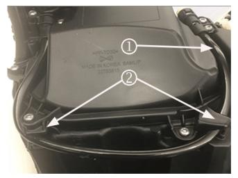
4. Detach the headlamp adjuster cable (1) so it is no longer trapped by the two retaining clips (2).
