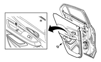
1. Remove the trim panel on the affected door. Refer to the appropriate Front or Rear Side Door Trim Replacement (Chevrolet) in SI.
