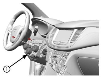
**Important:** Prior to final installation of the console and I/P trim, ensure smooth/proper operation of the temperature control knob by completing several rapid rotations of the knob.
