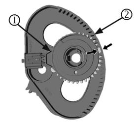
8. For proper alignment during installation, index the temperature valve gear (1) large female tooth to temperature control cable gear (2) large male tooth, as indicated by the arrows.
