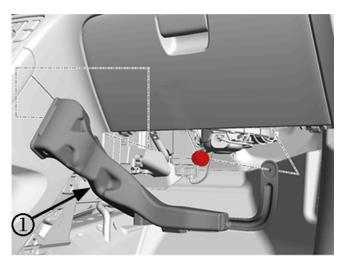
1. Remove the right side floor air outlet duct (1). Refer to Floor Front Air Outlet Duct Replacement - Right Side in SI.
