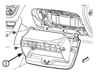
11. Install the I/P compartment. Refer to Instrument Panel Compartment Replacement in SI.
