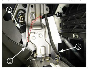
**Note:** To improve visibility of the cable and harnesses, a sheet of white paper was placed behind the tie bar in the graphic above. The cable end is also shown secured in position.
