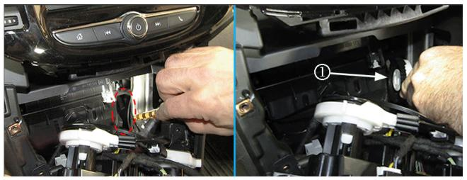
6. Start the routing of the new control cable by passing the cable pulley through the opening shown circled at the pointer in the graphic above. Pass the pulley through the opening, in the orientation shown (1) (with gear facing the driver side) and ensure the cable does not twist or kink during the routing.
