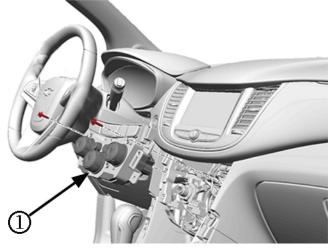
3. Remove the heater and air conditioning control with cable control (1). Refer to Heater and Air Conditioning Control with Cable Control Replacement in SI.
