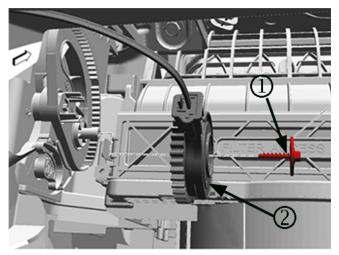
9. Install the temperature control cable retaining screw (1) and the temperature control cable (2) onto the heater and air conditioning evaporator and blower module. Tighten the screw to 2Y (18 lb in).
