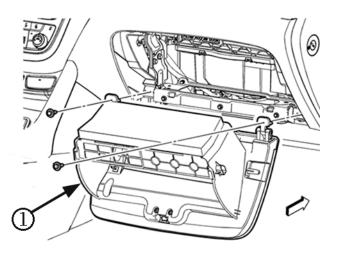
2. Remove the I/P compartment (1). Refer to Instrument Panel Compartment Replacement in SI.
