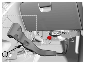
12. Install the right side floor air outlet duct. Refer to Floor Front Air Outlet Duct Replacement - Right Side in SI.
