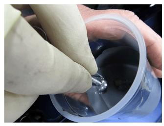
**5.** Prep the rivets by preparing a small portion of catalyzed primer in a mixing cup. Dip the end of the rivet in the primer OR apply a light coat of \*Lloyds Kryptonite Metal Treatment Part Number 36502 with a small brush.
