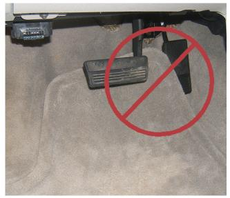
After installing floor mats, make certain they cannot move and do not interfere with the accelerator or brake pedals.
