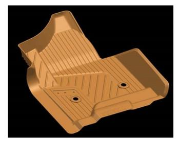
GM's carpeted and all-weather (rubber) floor mats, as shown above, are especially designed for use in specific GM vehicles. Using floor mats that were not designed for the specific vehicle or using them incorrectly may cause interference with the accelerator or brake pedal. Please review the following safety guidelines regarding proper driver's side floor mat usage with the customer.
