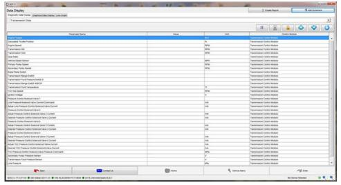
The Add Bookmark button can be highlighted before the road test by pressing the tab key until the button is highlighted or by clicking on the button.
