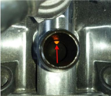
If the non return valve is not visible as shown in picture, then use a long cotton swab to wipe any excess oil from the valve to validate.
