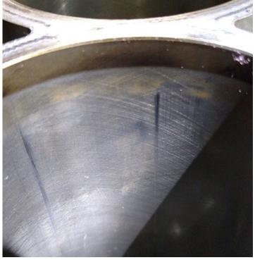
Shown below is an example of a damaged cylinder wall.
