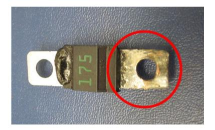
If the fuses show voltage stress is present, this is most likely the result of a poor connection. The Fuses are now available individually. If the entire fuse block needs to be replaced for any reason the fuse block includes both fuses.
