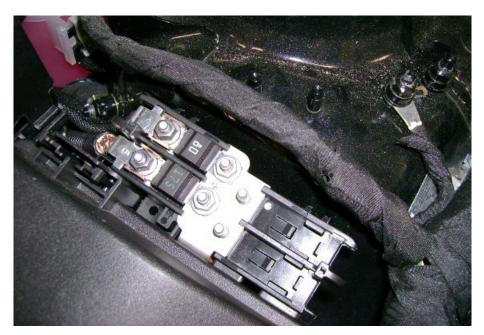
If the fuses pass inspection and they are not visually damaged in any way, install the fuses, carefully torque them to 4.7 Nm (42 lb-in), and re-evaluate the charging system operation. If the 175A fuse is open or has a poor connection, a P0A8F may be stored in history but the DTC may not consistently reset.
