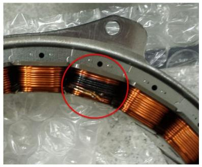
If no damage is found, replace all of the following parts: Motor 1 Position Sensor, Transmission Internal Harness, and Motor 1 Stator (damage may be on windings below the top layer). Replacing the Drive Motor Generator Control Module should only be ordered if the condition persists after replacing these parts.
