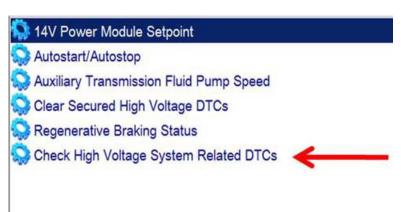
3) Now select clear the High Voltage DTCs in the HPCM and hit the reset button on the bottom of the screen. Wait 45 seconds before exiting the screen
