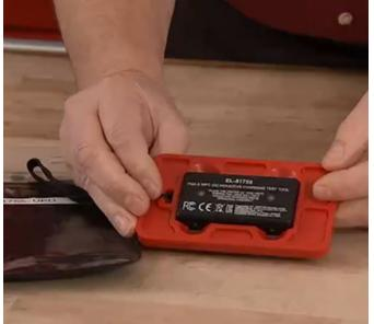
The EL-51755 Inductive Charging Test Tool can be used to verify charging system operation in a vehicle.
