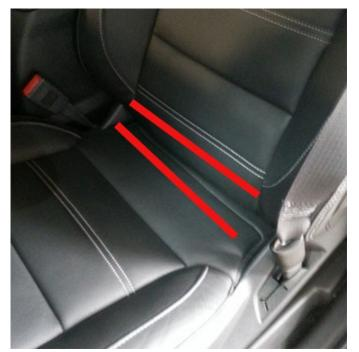
This concern could be caused by the seat bottom trim cover not installed correctly onto the cushion/foam, as shown below. If the seat cover is not completely and squarely installed onto the cushion/foam, it will give the appearance that the seat back is leaning or turned outward.
