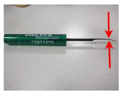
While looking down into the connector body at the terminals, there is a purple TPA that will align itself in the release position when the release tool is inserted into the release hole. Shown below is a shock terminal, that is already removed from the connector body, to show the metal locking tab (1) that will need to be pushed in with the terminal release tool before the terminal will pull out of the connector body.
