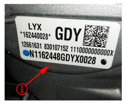
As shown in the above photos, the engine broadcast code can be found on the engine front cover or engine block below intake manifold
