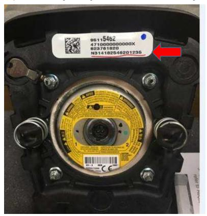
2014 Chevrolet Silverado & Sierra and 2016 Chevrolet Silverado & Sierra Replace the air bag instrument panel module. Refer to *Instrument Panel Air Bag Replacement* in SI.
