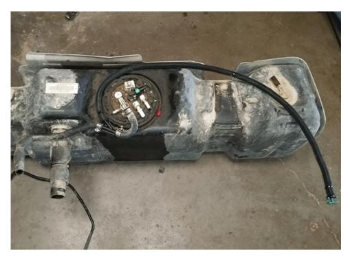
7. Remove the original fuel balance pump line from the pump tube (7) Refer to Plastic Collar Quick Connect Fitting Service. Doc Id# 2147646 and cross member (8) as seen below.
