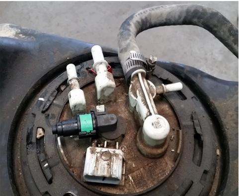
3. Measure the Fuel Tank Fill Vent hose  $5 \frac{1}{2}$ " from the end at the fuel pump module and cut with hose cutters as seen below (2).
