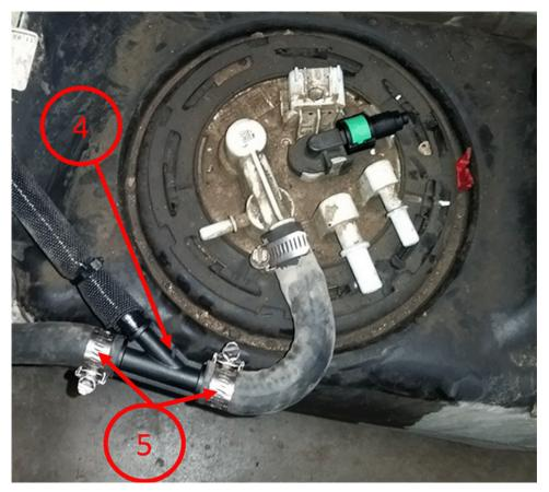
6. It is important to route the Vent Hose over the TOP of the fill hose as seen below (6) to prevent puddling of fuel in the line.
